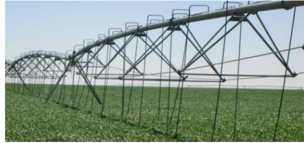
Figure 1b. LEPA irrigation typically applies water to alternate furrows through drag hoses directly to the ground surface, minimizing evaporation losses.
