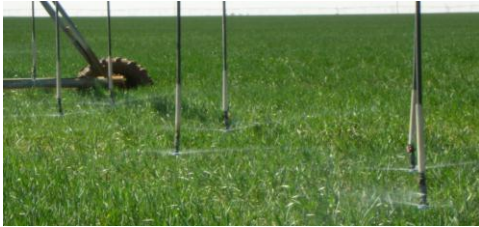
Figure 1e. Low pressure LESA spray nozzles deliver water near the soil surface and with large water droplet sizes to reduce evaporation losses compared to high pressure sprinkler systems.
