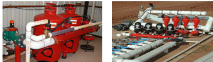
Figure 1h. Adequate filtration and maintenance are essential to longevity of subsurface drip irrigation systems.
