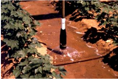
Figure 1c. Commercially available LEPA applicators are easily adapted between LEPA (bubbler mode, shown here) and spray mode.
