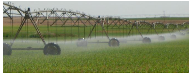
Figure 1f. LPIC and MESA apply water at low pressure, yet allow for application above (MESA) or within (LPIC) the crop canopy.
