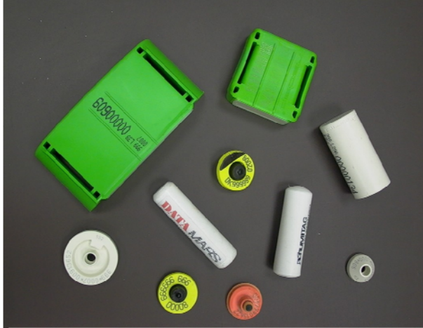
Figure 2. Examples of radio frequency identification tags (all meet the ISO Norm).
